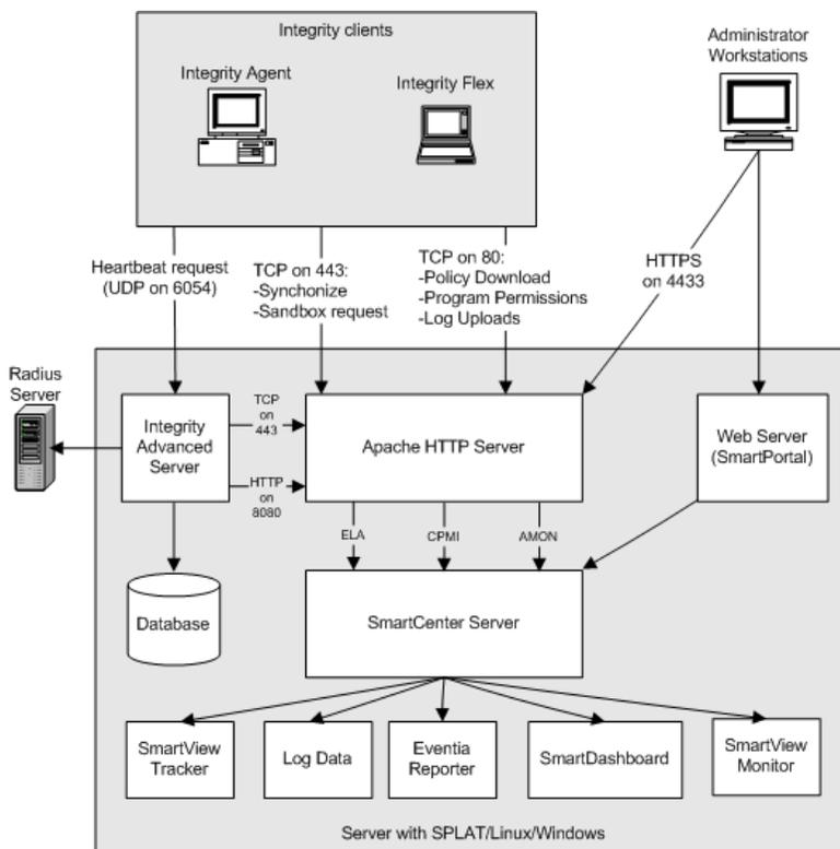
A typical Integrity Advanced Server configuration includes the following components:
